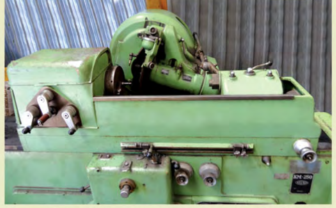
VİDA TAŞLAMA / SCREW GRINDING Ø 300 X 600
