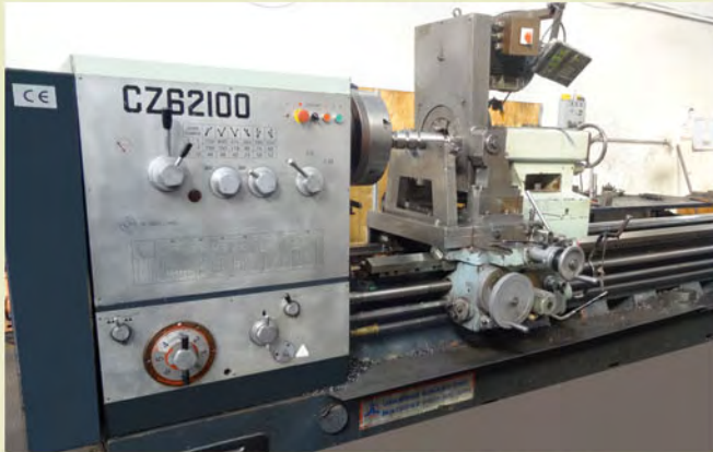
SONSUZ VİDA MAKİNASI / WORM SCREW MACHINE Ø 150 X 4000
