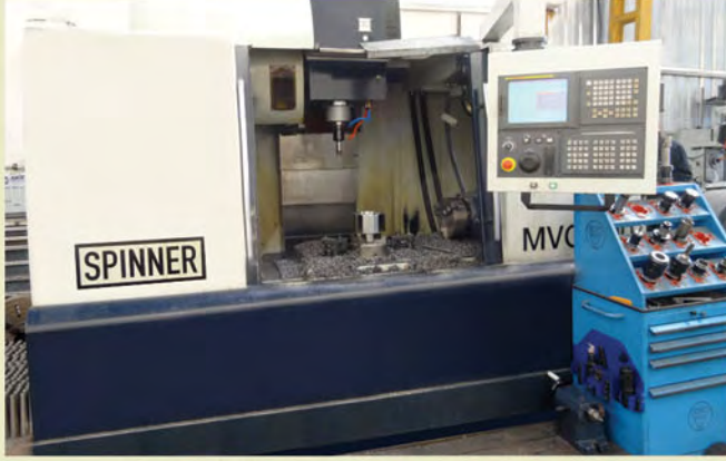
CNC DİKİŞLEME / CNC STITCHING X:1100 Y:600 Z:650 (4 EKSEN)
