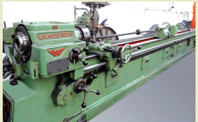
YATAY AZDIRMA / HORIZONTAL HOBGING MACHINE Ø 220 X 5000
